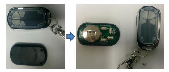
3. Push the battery out as shown in the picture below
