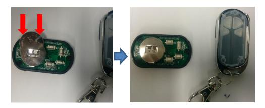
6. Put the remote back together by carefully placing the back part / circuit board on top of front side:
