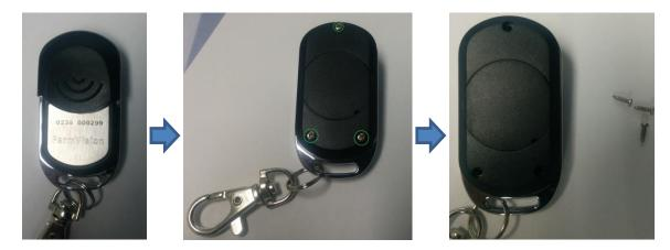
2. Carefully remove the top cover with the circuit board on.
