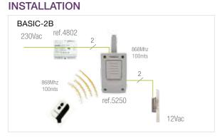
Stand-alone receptor powered by 12/24Vca/dc which allows for the management of up to 500 command codes RF 868Mhz. A channel (emitter button) can activate either of the two relays, or both simultaneously, in ref.5250. This allows the user to open pedestrian and vehicle gates by remote, from a distance of up to 100m. It can be programmed manually or by radio.
