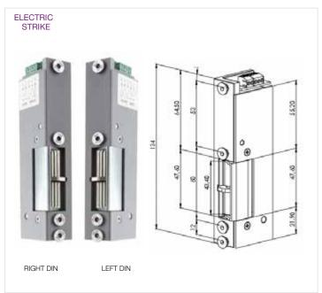
Door openers for security and emergency doors. It allows unlocking against pressures up to 450 kg. In addition, it incorporates a diode that avoids the electronic interferences and lengthens the life of the coil.
