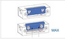
If the lock description contains MAX, it indicates that the latch is adjustable, allowing a perfect fit between latch and bolt in the lock, with a 4mm margin.
