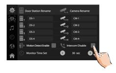
\*In default setting, intercom function is enable for the monitor.
