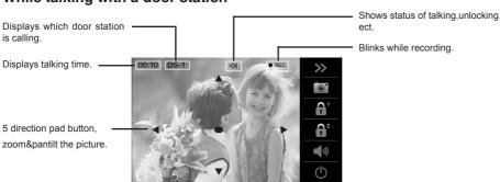
Note: The 5 direction pad operation should make effective with fish-eye door station.
