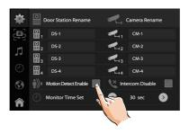
\*If this setting item has not been selected, the motion detect function is forbidden, and the Montion detect icon 🕅 🛚 will not display on main menu page.
