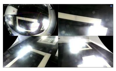
On a PTZ image, drag the mouse to rotate the image or use the scroll wheel to zoom in or out. A box appears on the fisheye image as the image rotates, and as you drag the box or move the scroll wheel on the fisheye image, the corresponding PTZ image rotates or zooms in or out as well.
